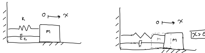
(a) A single degree of freedom harmonic oscillator, or SDOFHO for confusing and short.
